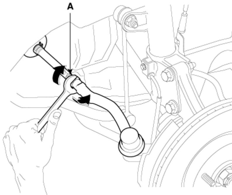
4. When completing the toe adjustment, install the bellows clip and tighten the tie rod end lock nut to specified torque.
