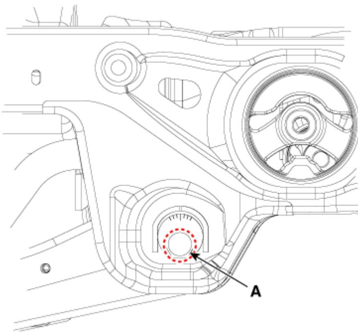
3. When completing the rear camber adjustment, tighten the nut to specified torque.
