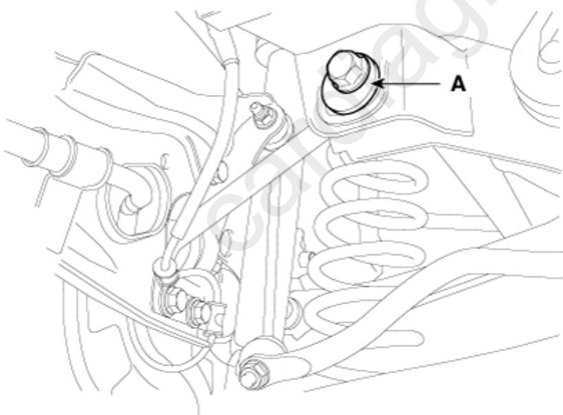
3. When completing the toe adjustment, tighten the nut to specified torque.
